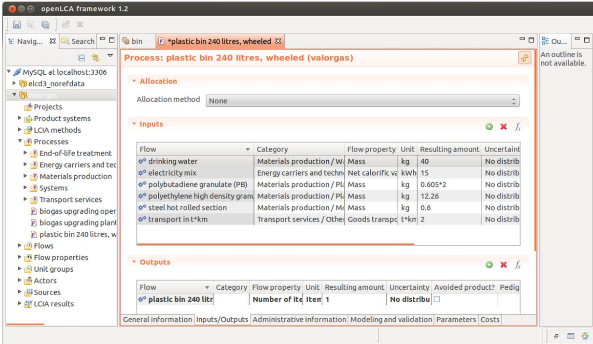
**Figure 10.** The new ILCD dataset 'plastic bin 240 litre, wheeled', generated in openLCA v.1.2.9 using the ELCD version 3 database. In total six flows serve as inputs for the model. The output is one 240 litre bin. Detergent for cleaning the bin during the life time was not modelled.
