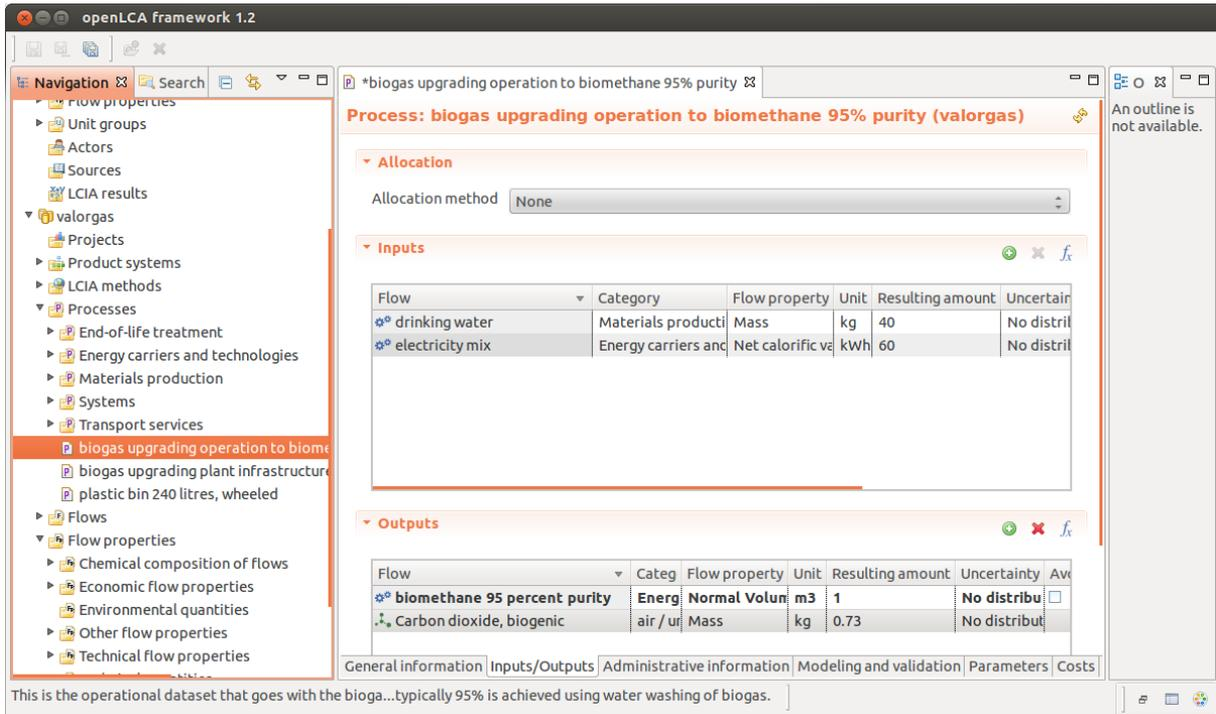
**Figure 6.** Metener gas upgrading operational process dataset in openLCA 1.2.9 using the ELCD version 3 database. Two inputs and two outputs are modelled
