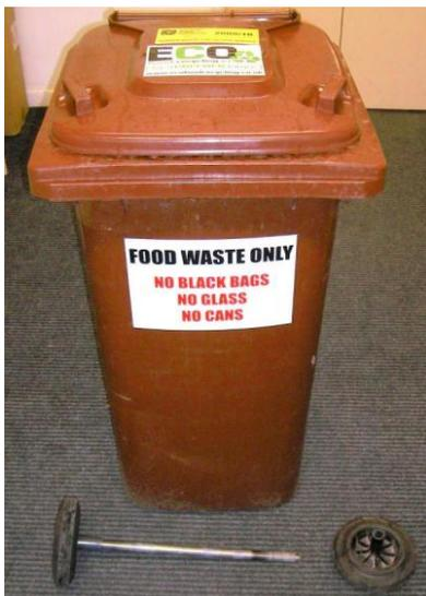
**Figure 7.** Standard 240-litre plastic bin, manufactured by SULO, used to store food waste in an institutional organic waste scheme. The bin was taken apart and parts were weighed.
